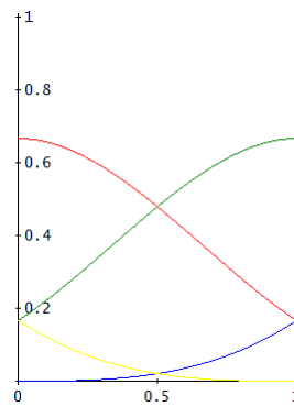
Figure 10.5 Degree 3 uniform B-Spline basis functions
